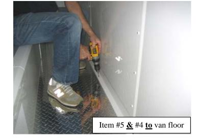
Be Sure Floor Is Square To Benches & Bulkheads. Attach Divider to vehicle. Pre-drill through floor(s) using 3/16" drill bit and attach using ½" x 1 ½" hex head lag bolts
